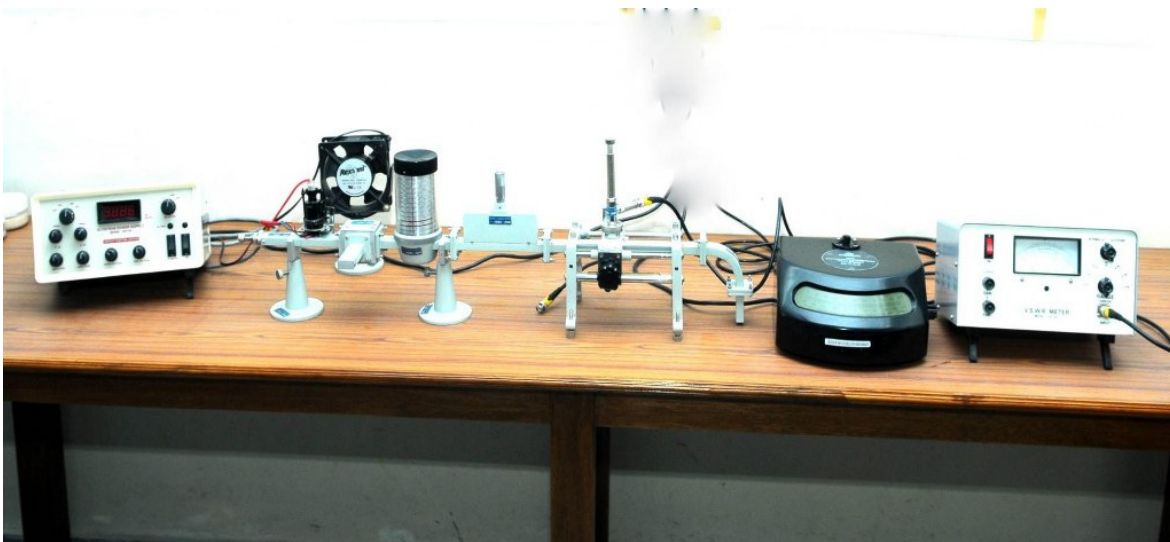
Experimental setup for determination of dielectric properties of food stuff in powder form by two point method
