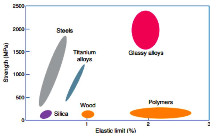
**Figure 1.** Metallic glass alloys combine higher strength than crystalline metal alloys with the elasticity of polymers [8]
