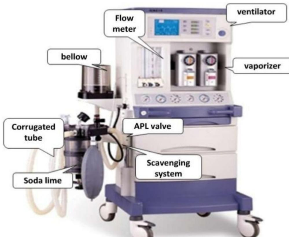
regulator. Intermediate pressure areas (37-50 psi) consist of just after regulator to flowmeter. Low pressure areas (0-30 cm of water) from flowmeter to common gas outlet. Cylinders are colour coded according to the gas of the cylinder contains. Tag label indicates whether the cylinder is full, part full or empty.
