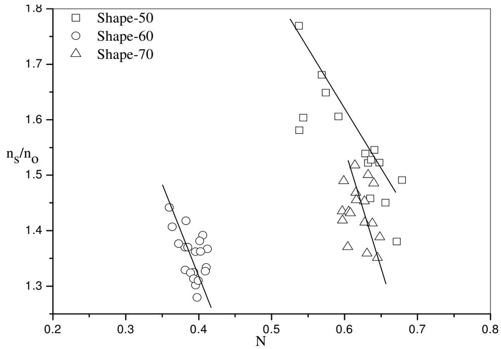
**Figure 3: Variation of Manning's roughness coefficient with N (slope-0.00116)**
