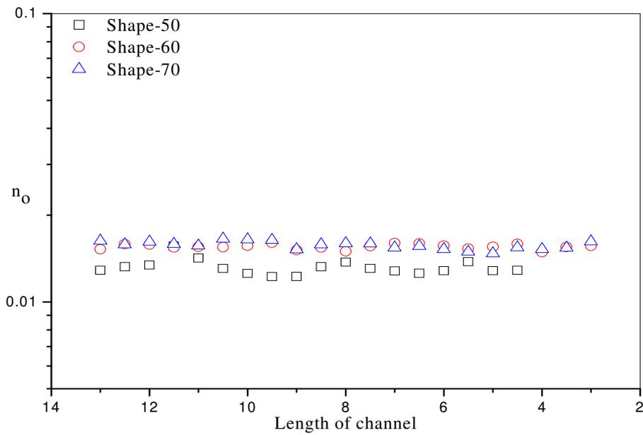
**Figure 2: Variation of Manning's roughness coefficient without seepage (slope-0.00116)**
