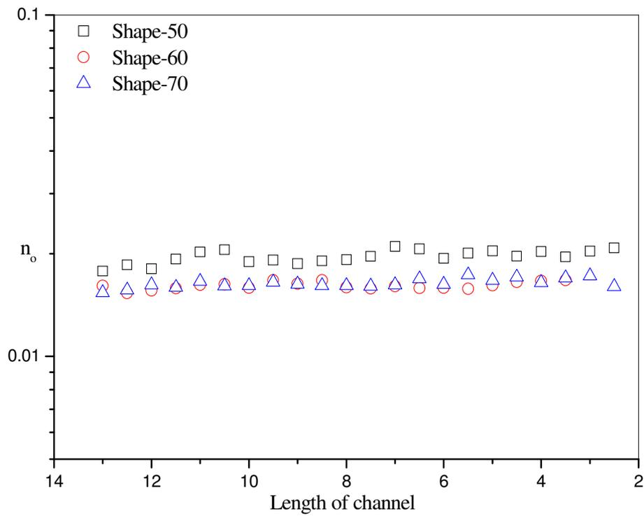
**Figure 4: Variation of Manning's roughness coefficient without seepage (slope-0.00249)**
