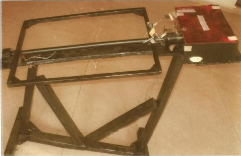
Figure 3. Photograph of the Implemented Automatic Solar Insolation Tracking System
