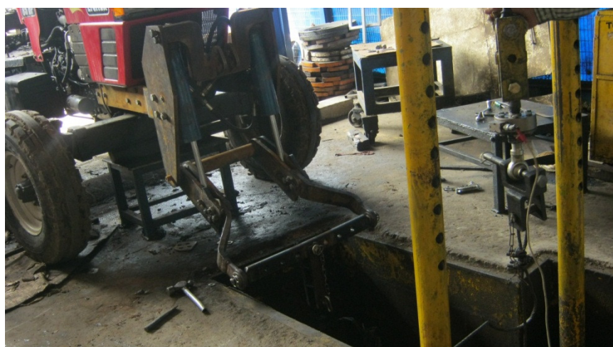
Fig. 9. Lift capacity measurement at lower hitch point.
