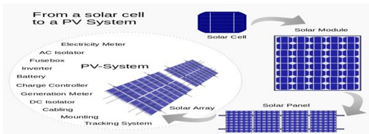
Fig: 2- Solar cell to PV system diagram <sup>[18]</sup>
