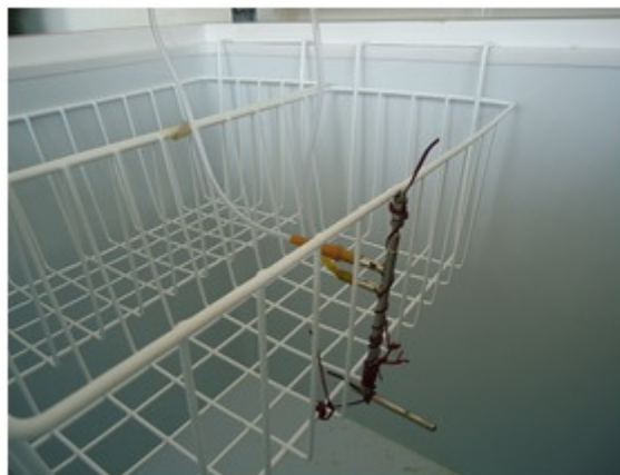
Figure 3. Pitot tube arrangement for air velocity measurement.
