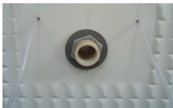
Figure 5. Arrangement for inserting thermocouples and for tubes for air velocity measurement
