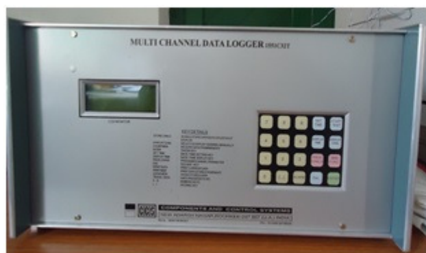
Figure 4. 32-Channel data logger system for temperature measurement
