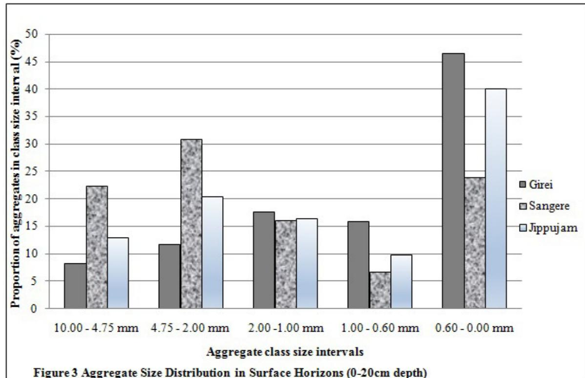
Figure 3 Aggregate Size Distribution in Surface Horizons (0-20cm depth)
