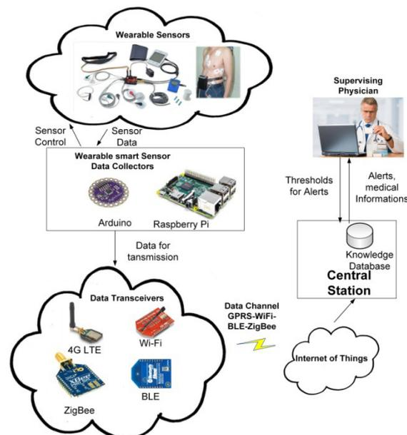
A WHMS is developed based on wearable sensors to exchange patient data with a Central Station. The data transmission is performed using services over existing wireless technologies (3G/4G or Wi-Fi) and protocols.
