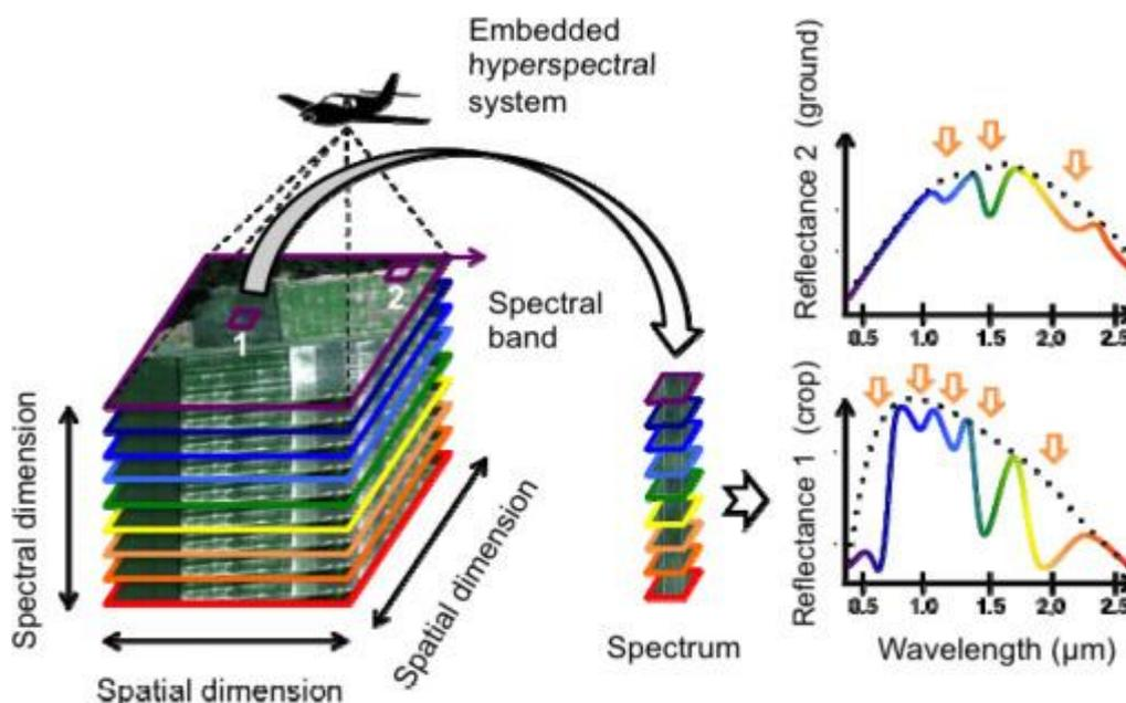
**Fig 1 Spectral and Spatial dimension of Hyperspectral Imaging**
