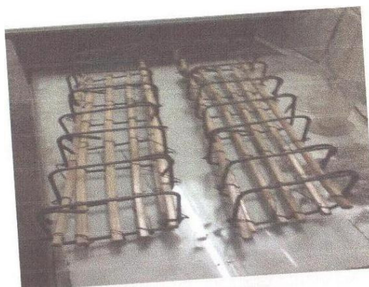
Fig. 1: Bamboo reinforcement with steel stirrups
