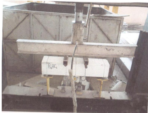
Fig. 2: Testing of beam under two concentrated loads
