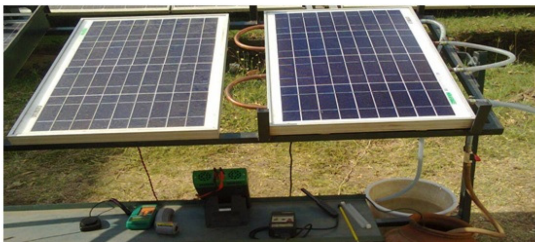
Fig 1: Experimental setup of PV and PV/T system
