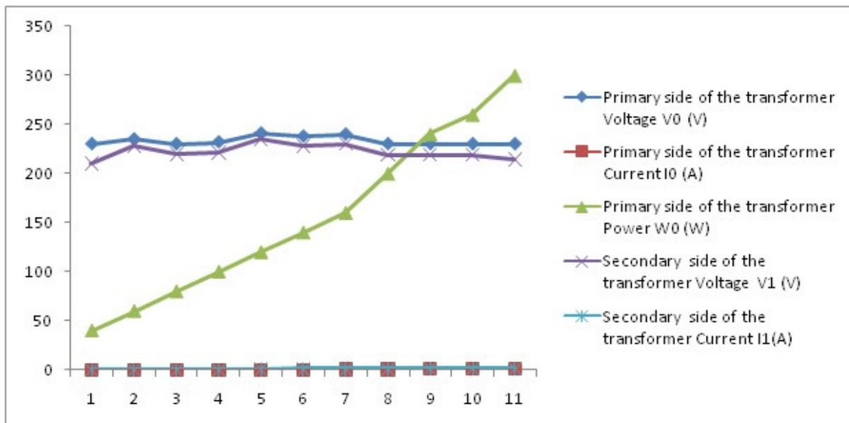
Fig.3. Demostation of primary and secondary current voltage and power characteristics
