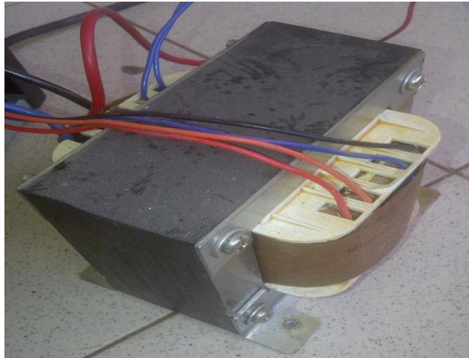
**Fig.1.** shell type transformer
