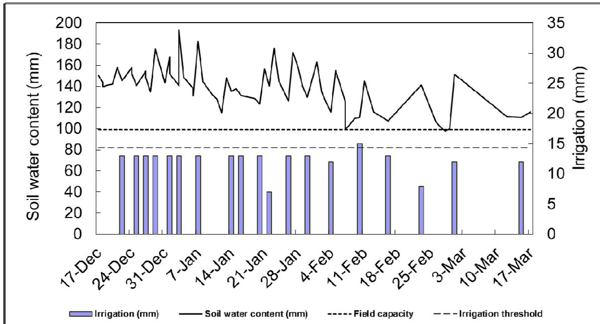
**Figure 6. Soil water content measuring in the soil profile in location T3 with a Diviner 2000 calibrated per depth**
