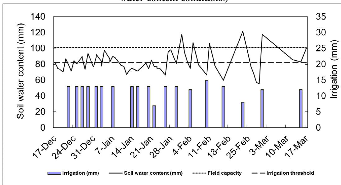
**Figure 4. Soil water content measuring in the soil profile in location T1 with a Diviner 2000 calibrated per depth.**
