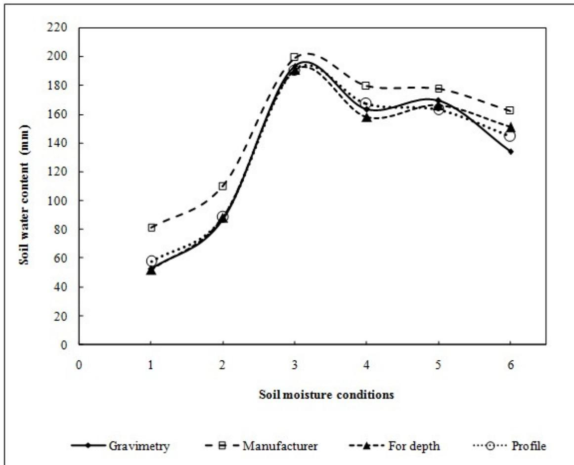
**Figure 3. Soil water content estimates (mm) from different calibration equations (manufacturer, per depth, soil profile) and the actual soil water content determined by the gravimetric method from the six reading points evaluated (two reading points per water content conditions)**
