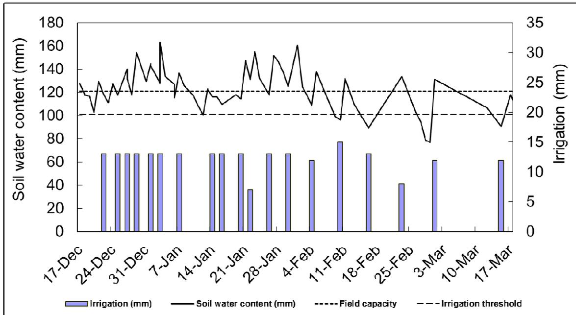
**Figure 5. Soil water content measuring in the soil profile in location T2 with a Diviner 2000 calibrated per depth**
