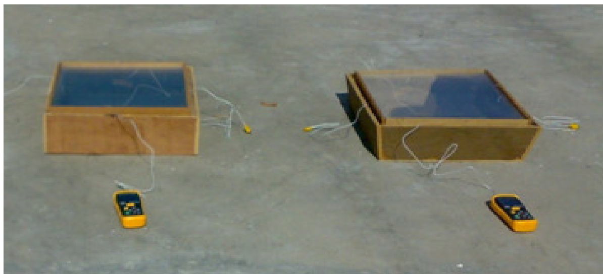
Fig. 1. Cuboid and trapezoidal hot box solar cookers with thermocouples and digital temperature indicators.
