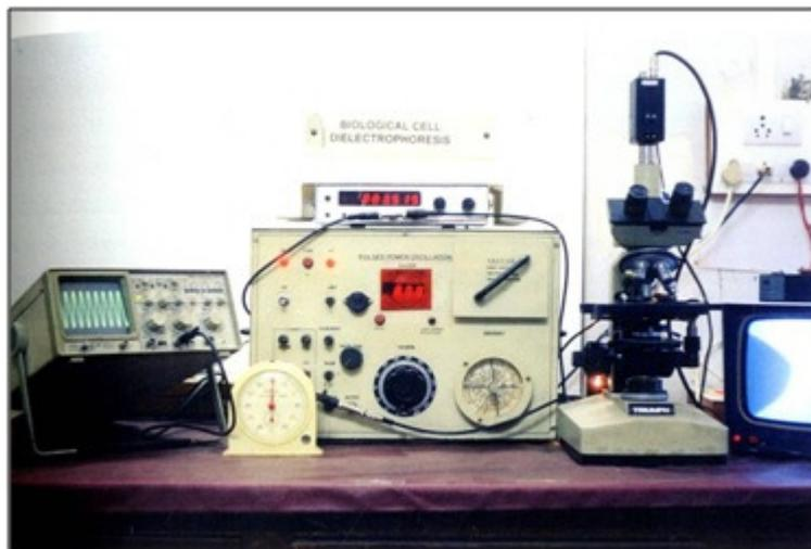
**Fig 3.** Dielectrodynamic setup
