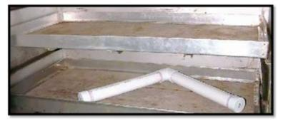
After assembling the PVC pieces, and allowing the glue to dry (12-24hr), place the entire assembly into a  $120 - 135^{0}$ C oven for 5-10min. Keep checking the pipe by squeezing it until
