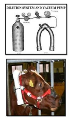
After the sampling collection period has been completed, the canister taken off the animal and connected to the dilution system and the final pressure recorded. Nitrogen is then slowly added until the pressure in the canister is increased to about 1.2 ATM. Another pressure
