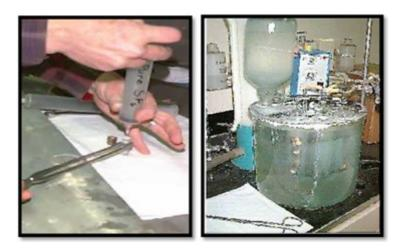
The tube should then be placed in a glass receptacle, in a 39°C water bath. A small flow of clean  $N_2$  gas is maintained to purge the glass receptacle of SF6 emissions. Weights of each tube should be taken weekly to determine the release rate of SF6. Five to six weeks is generally required to gain a goof idea of the release rate.
