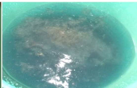
Figure 5. Disintegrated filler sheet in water
