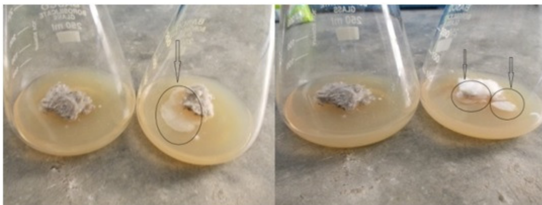
Figure 3. Growth of fungi in on test control and commercial product's filler (shown by arrows) and in gel treated samples (left, in both images), AATCC 30:1993 Testing of Developed Napkin (IS: 5405-1980)
