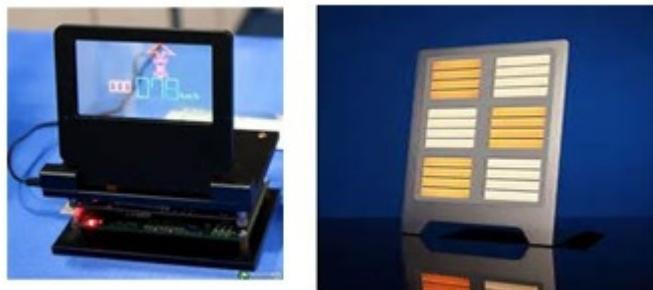
**TRANSPARENTOLED** (LG image) **TOP EMITTING OLED** (leds magazine)
