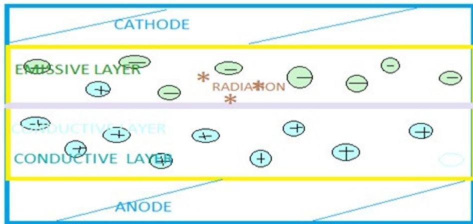
The working of OLEDs is more-or-less similar to LEDs but the number of layers sandwiched in OLEDs bring about a difference all around. The anode and cathode are directly connected to the supply. These layers provide electrons and holes respectively. The conductive layer becomes positively charged and the emissive layer becomes negatively charged as the power is applied. Due to the electrostatic force applied the electrons (negatively charged particles) move from the conductive to emissive layer.
