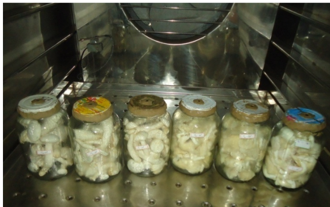
Fig. 1 Respiration study of mushrooms placed inside the humidity chamber
